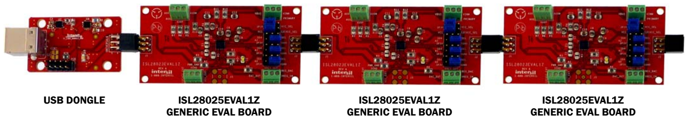
FIGURE 9. PICTURES OF SEVERAL ISL28025 GENERIC BOARDS CONNECTED TO A DONGLE ENABLING SYSTEM VIEW
